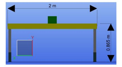
Dimensions are also automatically aligned to face towards the nearest axis that the camera is looking along. Dimension text can be flipped by pressing the Alt Key during the positioning of the dimension. The View Cube can be used to align the view precisely to any given axis/plane.
