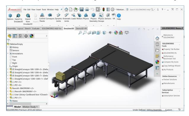
The CAD model marked up with Aspects can be Exported to Emulate3D where it can be simulated and connected to a PLC to test control logic.
